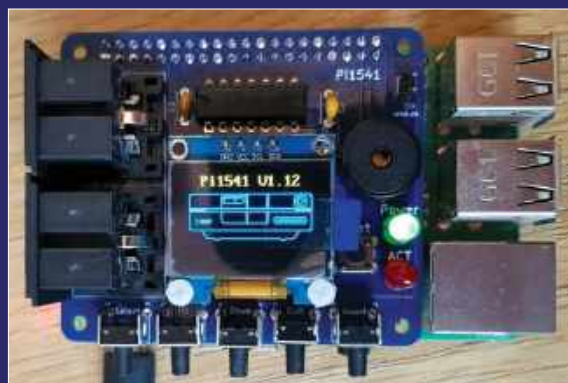
There are a few different Pi1541 designs on the market. This one comes with a rather fetching OLED display too.
