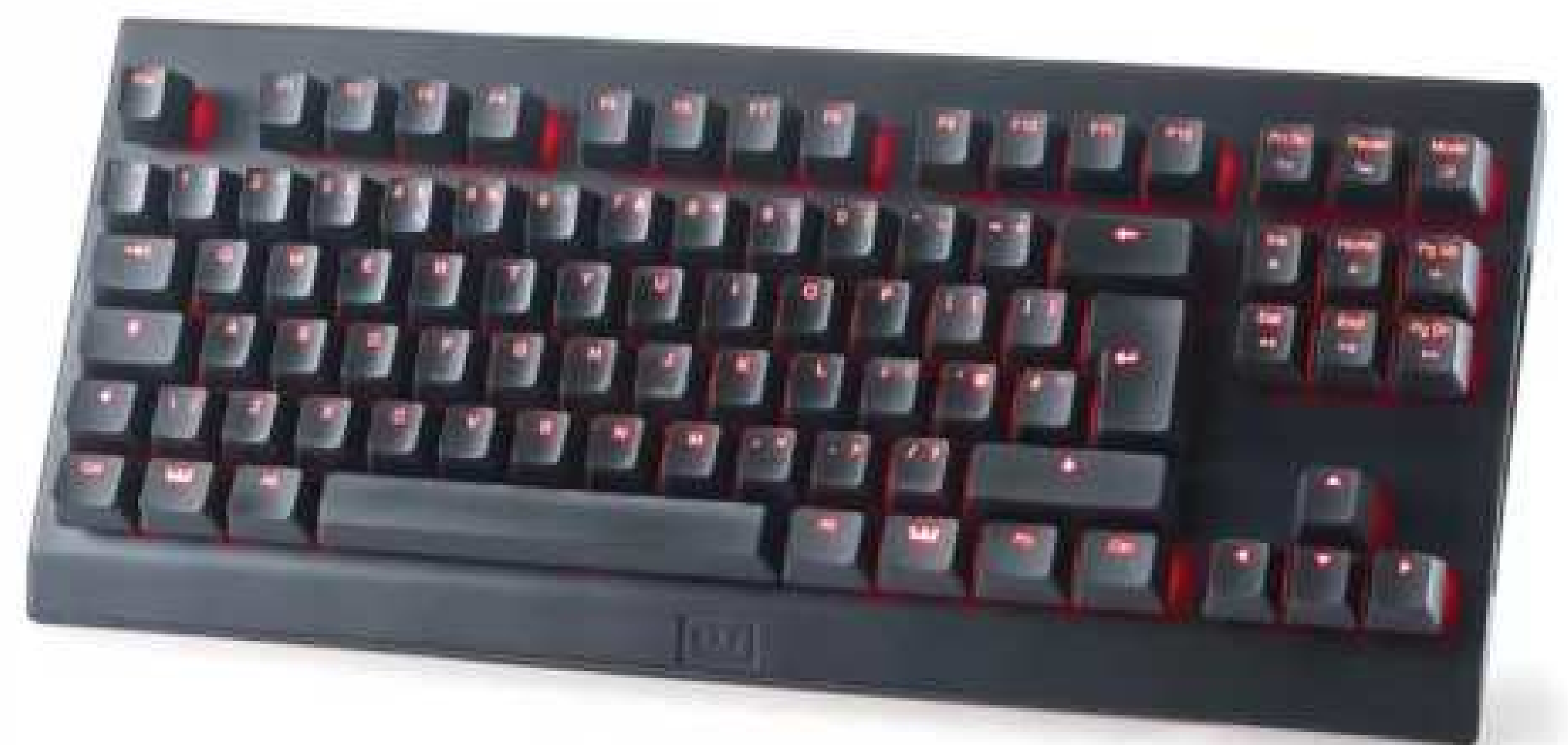
One of the first to break into the mainstream with optical keyswitches, Wooting's One keyboard was a phenomenal piece of kit.
