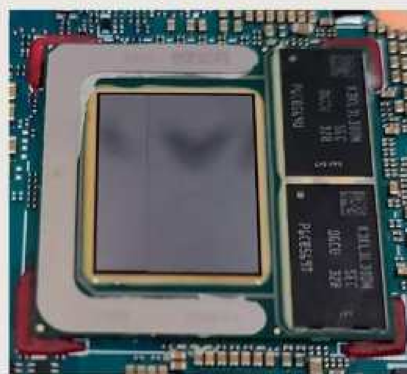
Lunar Lake consists of a compute and platform controller tile by TSMC.
