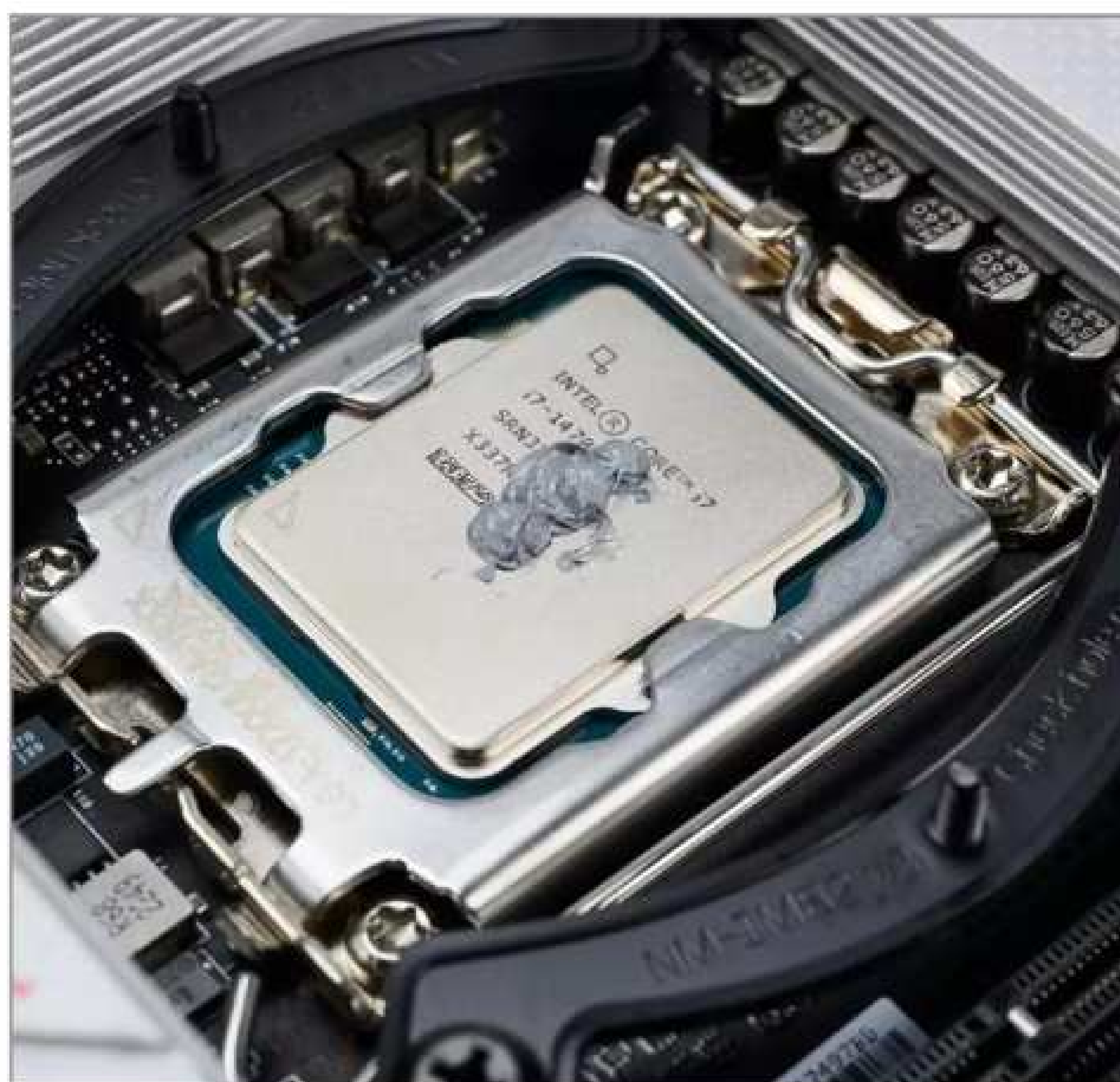
Our master builder Zak Storey says to use a thin strip of thermal paste down the middle of the CPU.
