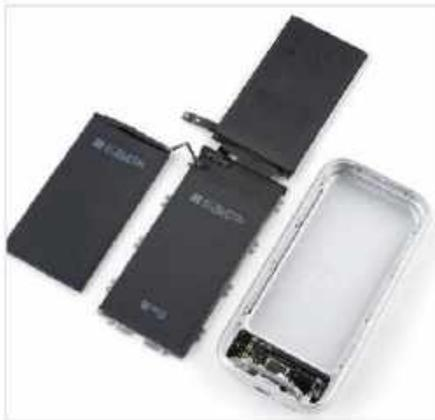
**Far left: The glass panel is glued on. It didn't break, but its protective plastic film got a little peeled up and a bit melted.**
