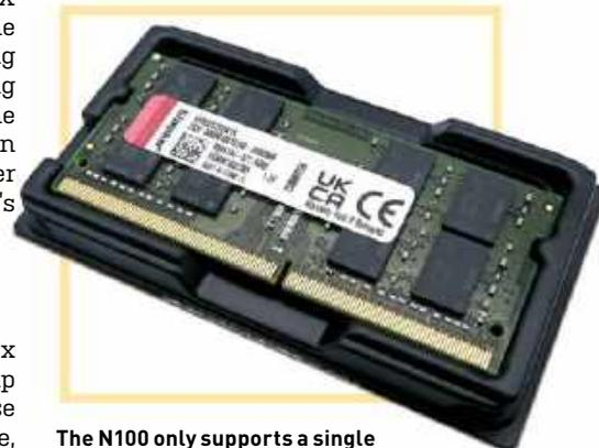
**The N100 only supports a single stick of SO-DIMM DDR4 RAM.**
