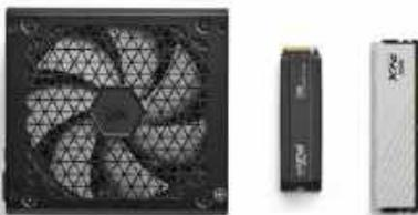
**[37] OPTIONAL SPARE HARDWARE** If you have hardware lying around from older builds that's compatible with what you're working on, it can be valuable. For instance, if you've got a Z790 board, but it hasn't been flashed ready for that new 14th gen chip, a 13th gen processor is useful. Likewise, memory kits for memory diagnosing, SSDs, or even power supplies can help you out, and make diagnosing system faults easier.
