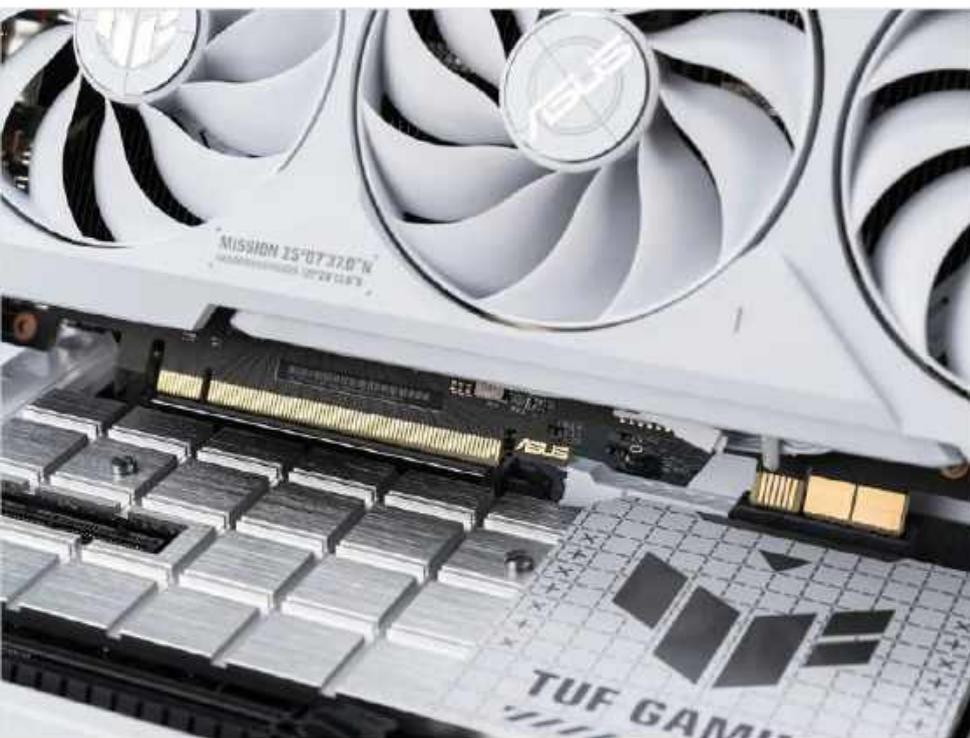
All the power being delivered by a custom PCIe slot legitimately sounds brilliant—let's get rid of pesky GPU power cables.
