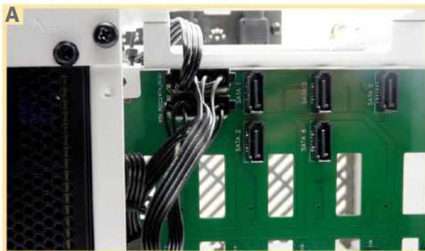
**Connect the PSU's twin Molex connectors to the SATA backplate.**
