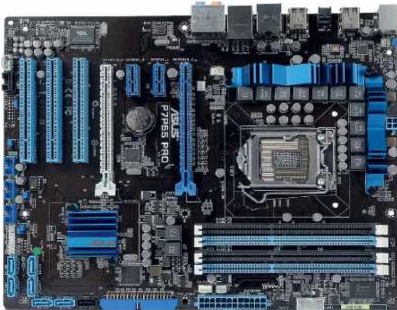
Socket LGA1165 with support for Intel 'Clarkdale' processors was the first time Intel included graphics on the same die as the CPU.
