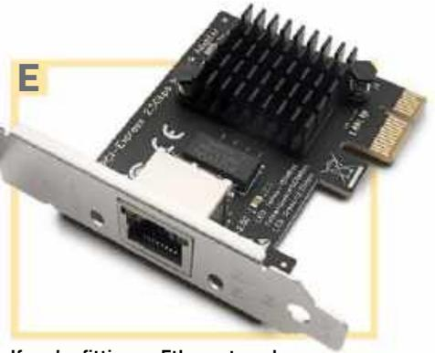
If you're fitting an Ethernet card, don't forget the low-profile bracket.
