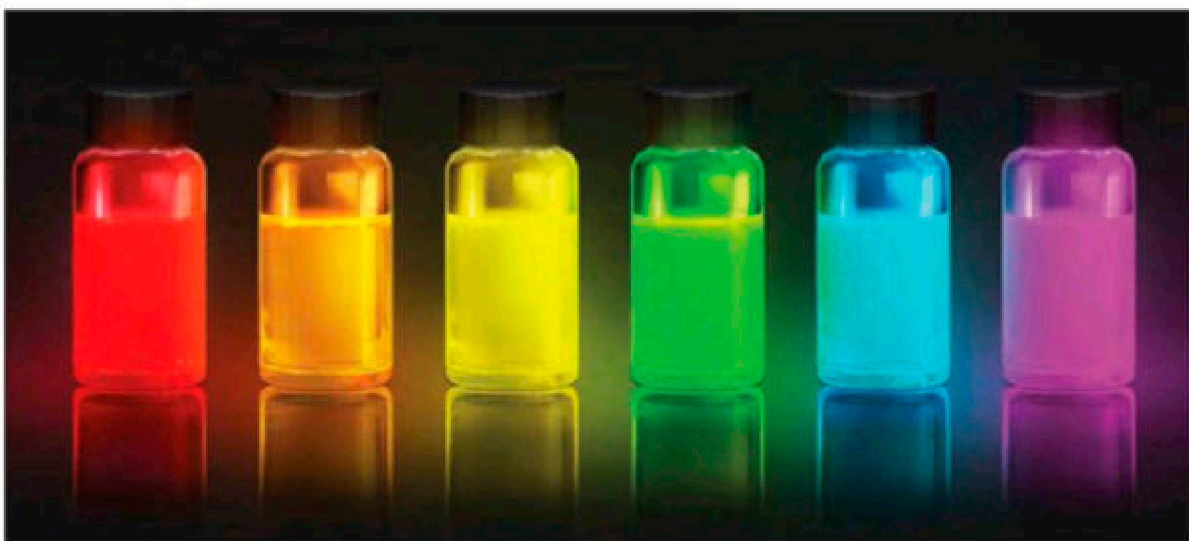
FIGURE 5 Suspensions of quantum dots of different sizes glowing under ultraviolet light
