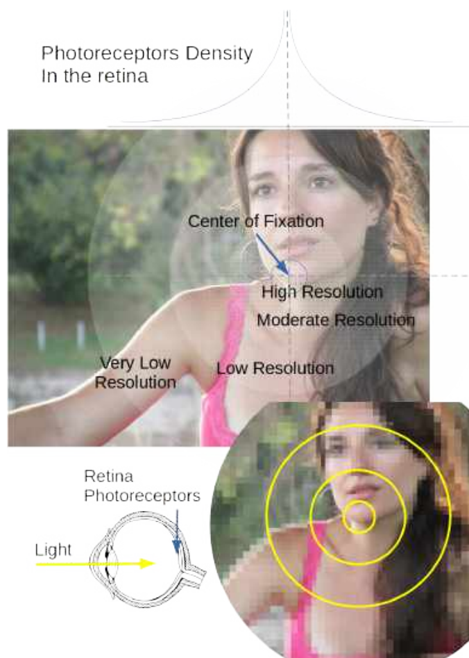
Fig. 1. Foveation in biological agents is a phenomenon in which the density of photoreceptors located on the eye's retina varies in a way that there is acutely more density near the fovea, while such a density decreases drastically in the fovea's vicinity. The fovea, is a small fraction of the retina which corresponds to the center of fixation in the sight. The consequence is that the perceptual detail regarded by the agent varies across the image according to the current fixation point, which confers the highest resolution region of the image to the center of the eye's retina, ( i.e. the fovea)
