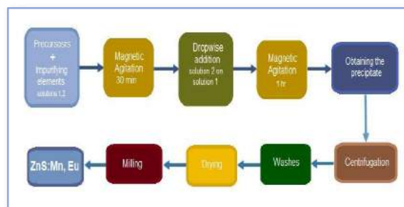
Fig. 2. Synthesis of ZnS Nanoparticles doped with Mn and Eu
